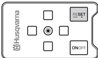
The surrounding red LEDs indicate which direction the machine must be angled to achieve the required position.
