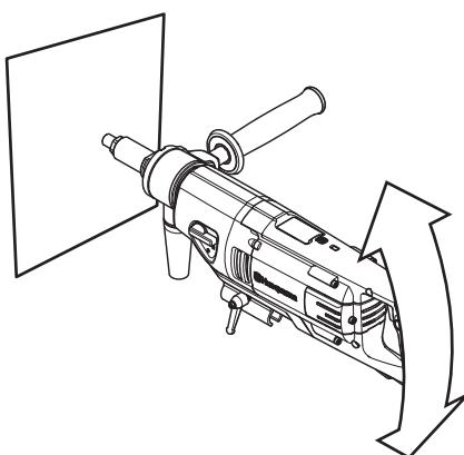
If the back of the machine is tilted downwards, the central green LED goes out and the front red LED lights up. If the back end of the machine is tilted up, the back red LED lights up.
